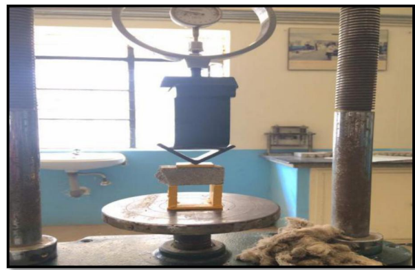
Figure 2 : Shear strength test in progress
