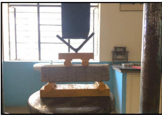
Figure 1 : Flexural strength test in progress
