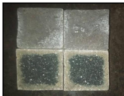
Figure 4: View of specimens showing Chloride Penetration
