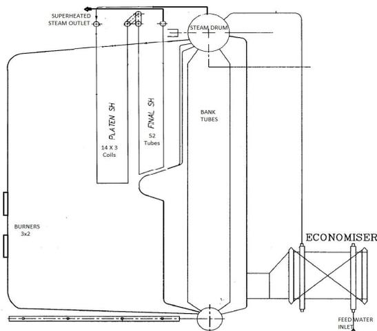
Figure 1. Schematic View of the Boiler.
