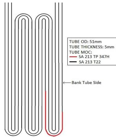
Figure 2. Schematic View of the Platen Superheater.
