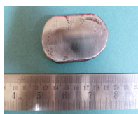
Figure 1 Typical as cast ingot (9Cr1Mo-12Zr-4 NMFP) MWF alloy
