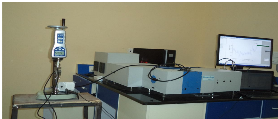
Fig.3: Test set up to measure TL intensity of phosphor under compressive/ tensile load
