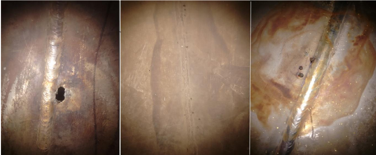
Severe pitting observed near the weld joints as well as parent metal of CBD vessel
