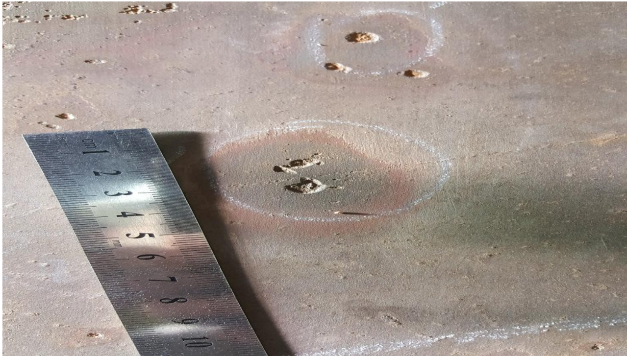
Figure 6: Deep Pits along with Mechanical Damages
