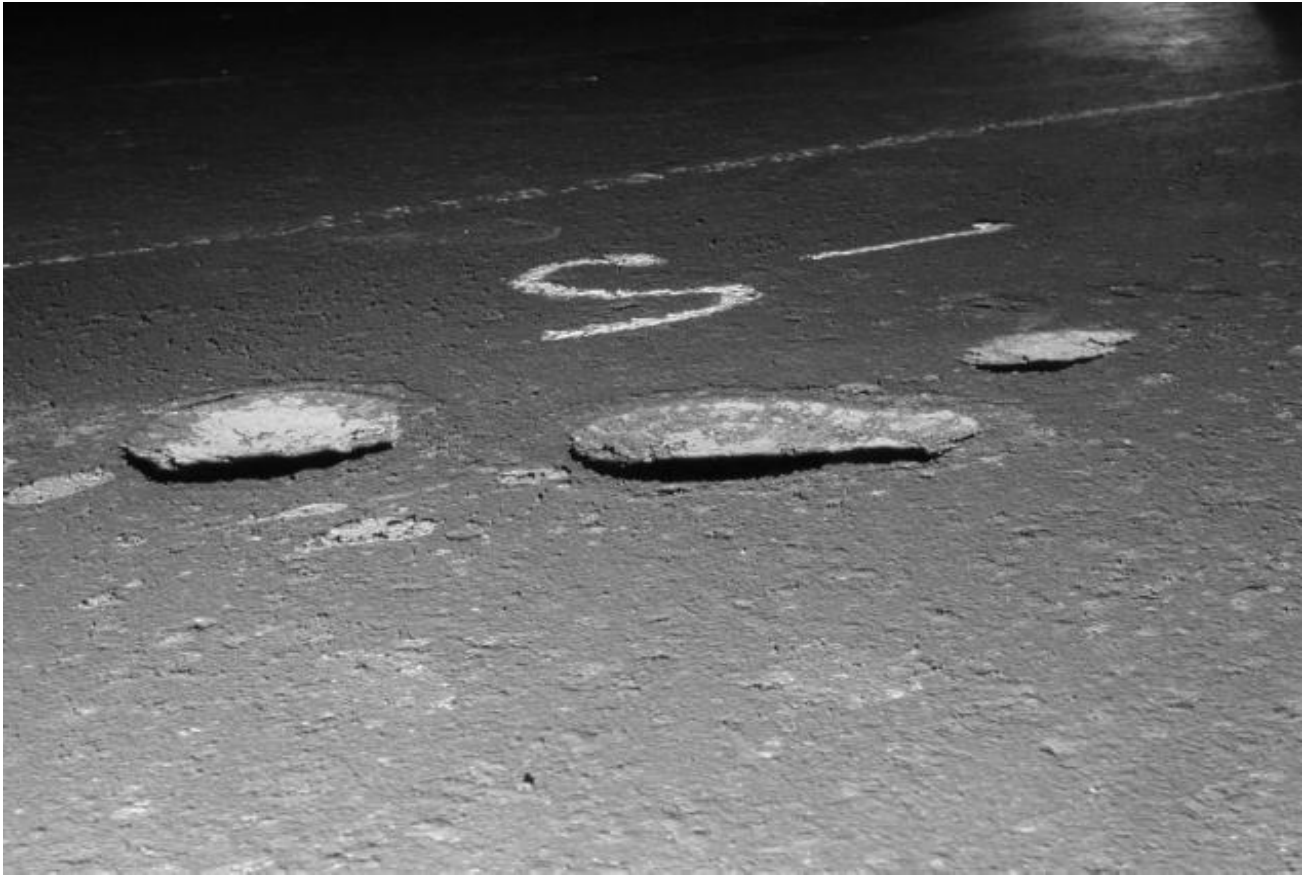
Figure 1: Pitting on the Bottom Plate of Storage Tank due to MIC
