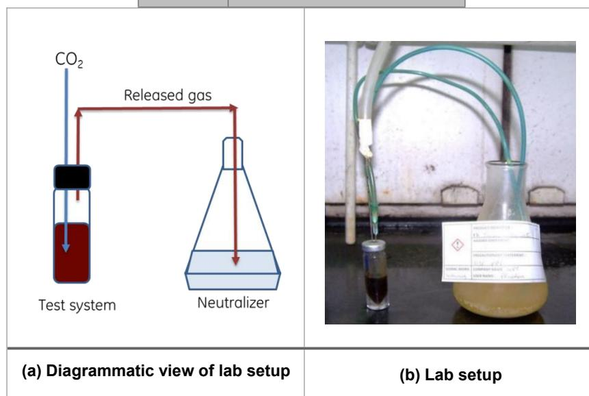
**Figure 1: Gunk test setup**
