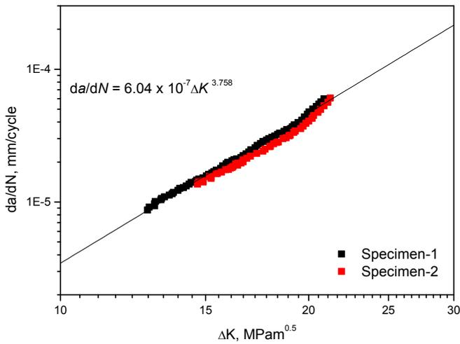
**Fig. 7: The test curves for da/dN**
