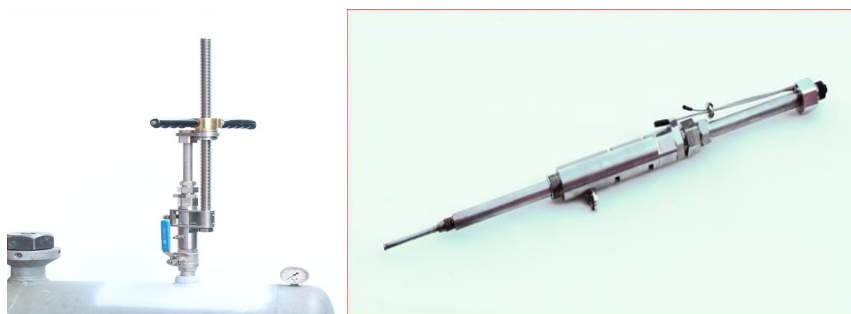
Fig 1: A Retractable (moderate pressure, high temperature) ER probe (right), and probe installed with retractor tool through packing gland and full bore valve (left).
