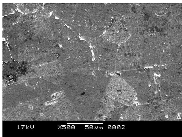
**Figure 7 Microstructure of Cross-Section near Outer Surface at Mag-500x**
