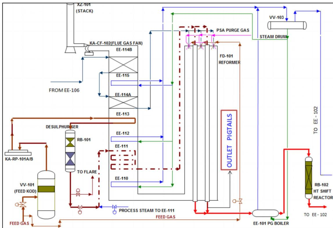
Figure 1 Process Flow Diagram of Hydrogen Reformer Section
