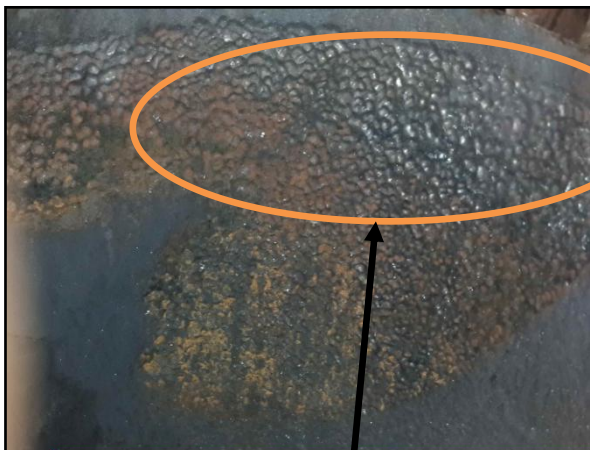
Fig 2(a). Metal loss in the form of small bubbles on the internal surface of pipe
