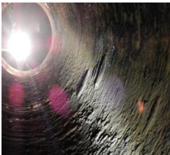
Figure 2 and 3: Blister on shell ID
