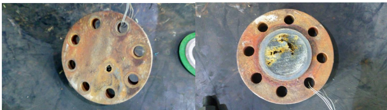
Figure 5: Failed end blind – External surface (left); internal surface (right)
