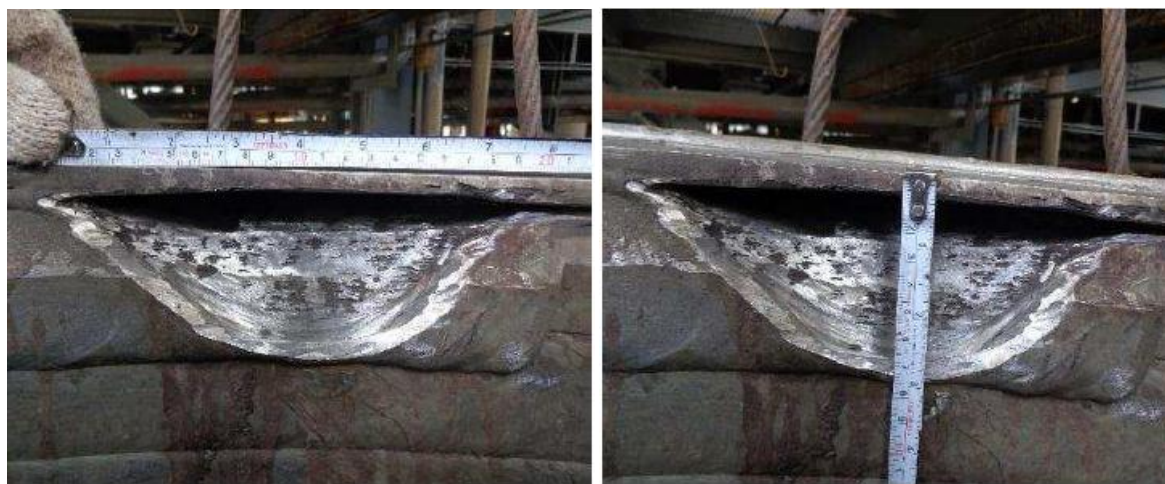
Figure 4: Extent of metal loss in the underlying base material under the overlay
