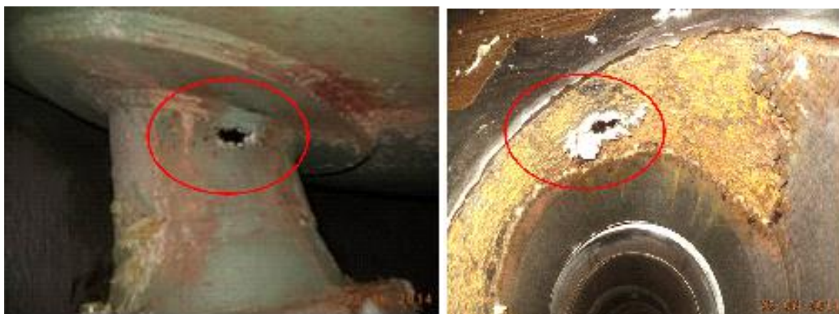
Figure 1: Failed nozzle: Left – view from Outer diameter; Right – view from Inner diameter
