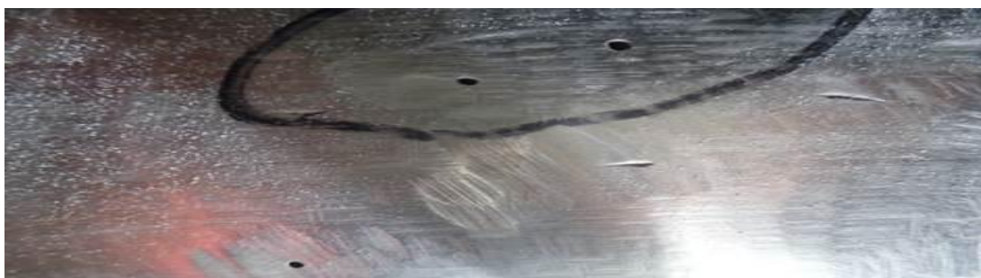
Figure 2: Pits in the circumferential seam weld overlay
