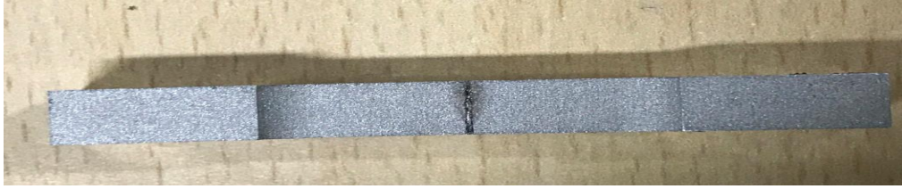
Figure 5: Side view of the fatigue specimen used for short fatigue crack studies. A sharp crack is generated on one edge of the specimens using precision laser cutting on a micro-machining center. Crack thus generated has approximately 100 \mu\text{m} width and 1 mm initial length.
