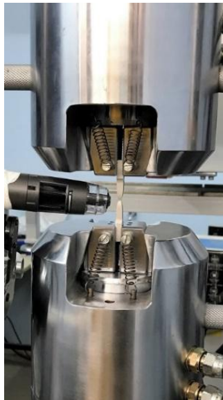
Figure 6: High resolution digital microscopes used for tracking the propagating short fatigue crack
