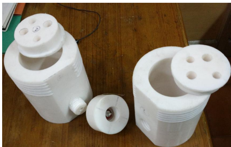
Figure 3: An In-house fabricated Devanathan-Stachurski cell shown in the disassembled configuration. Among the three compartments shown, the middle one holds the metal specimen exposing both its surfaces to the electrolyte in the right and left compartments those being the galvanostatic and the potentiostatic side of the cell.
