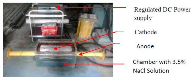
**Figure1 Experimental set –up to corrode the tubular compression members under unstressed condition**
