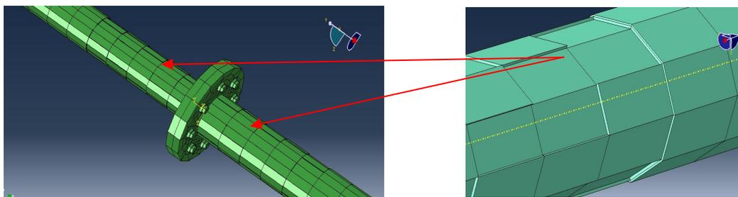
**Figure 9** simulation of combined effect of uniform and pitting corrosion effect
