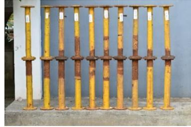
**Figure 5** Experimentally observed deformed profile of tested members
