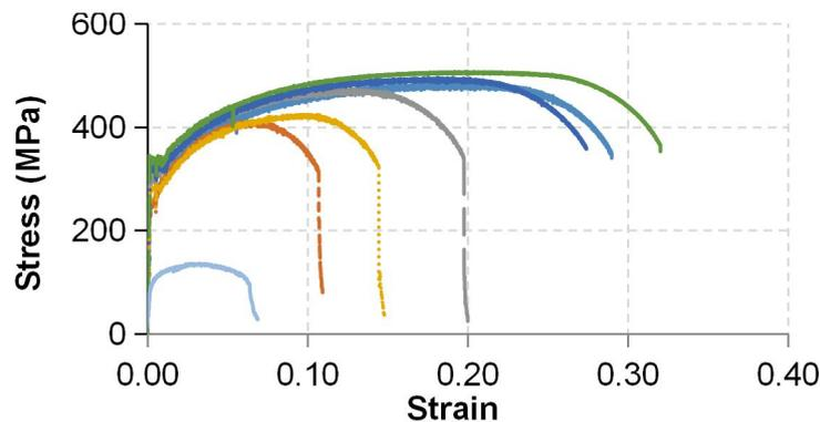
**Figure 3** Stress vs. strain behaviour of corrosion induced and uncorroded steel samples extracted from tubular members.
