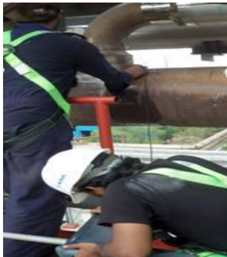
Figure 3: PAUT for detection of thermal fatigue crack at hydrogen quench line Of OHCU Reactor effluent line
