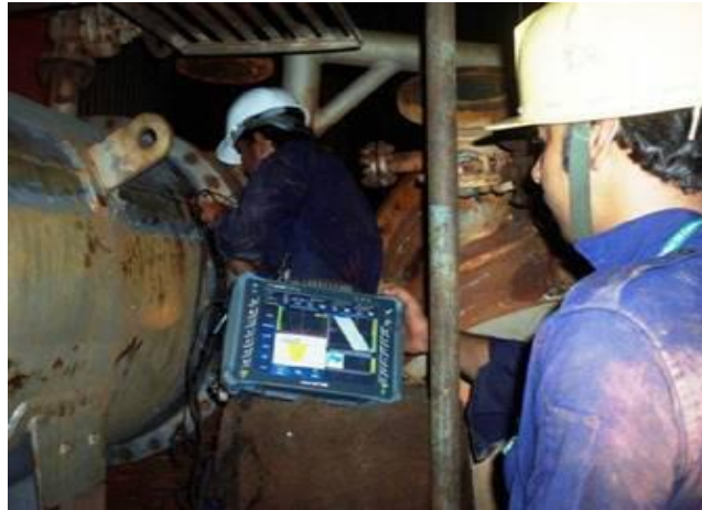
Figure 4: PAUT for detection wet H 2 S cracking
