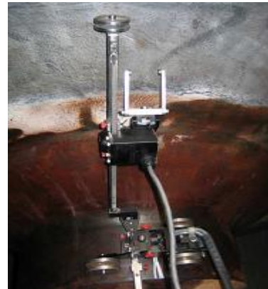
Figure 7 & 8: Above images show scanner and probe placement for PAUT examination
