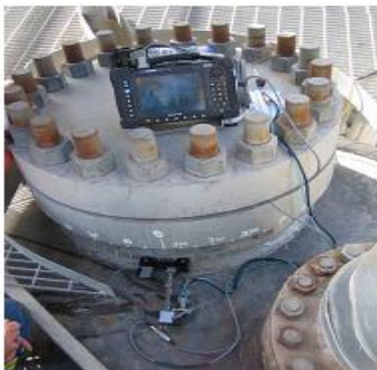
Figure 7 & 8: Above images show scanner and probe placement for PAUT examination
