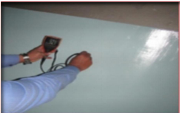
Figure 5: View of DFT Test readings taken in accordance with NACE SP 0188 [5]
