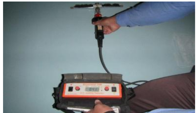
Figure 6: View of Holiday Test in accordance with SSPC PA 2 [5].
