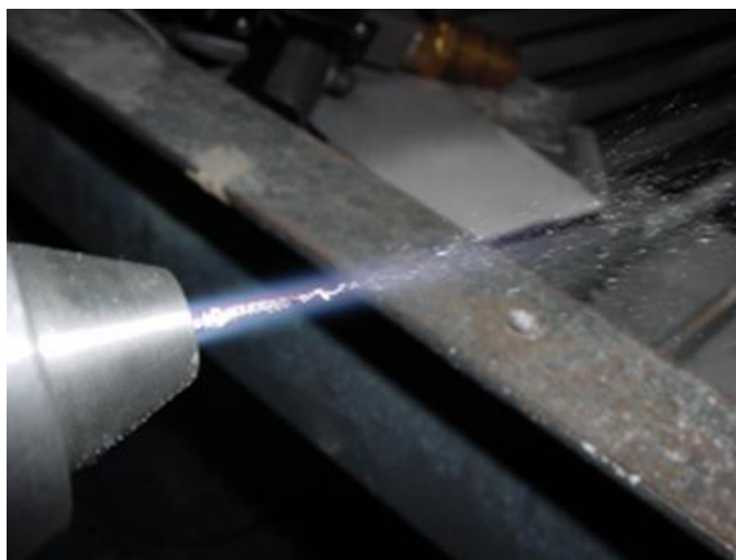
Figure 1: Thermal spray coating by using aluminum metals
