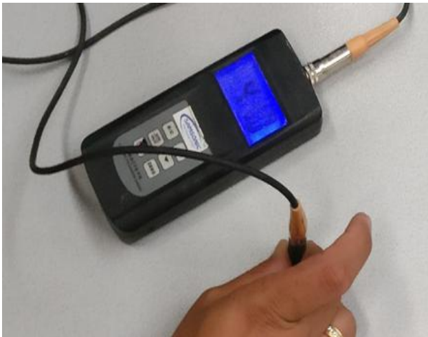
Figure 2: TSA coating thickness check test
