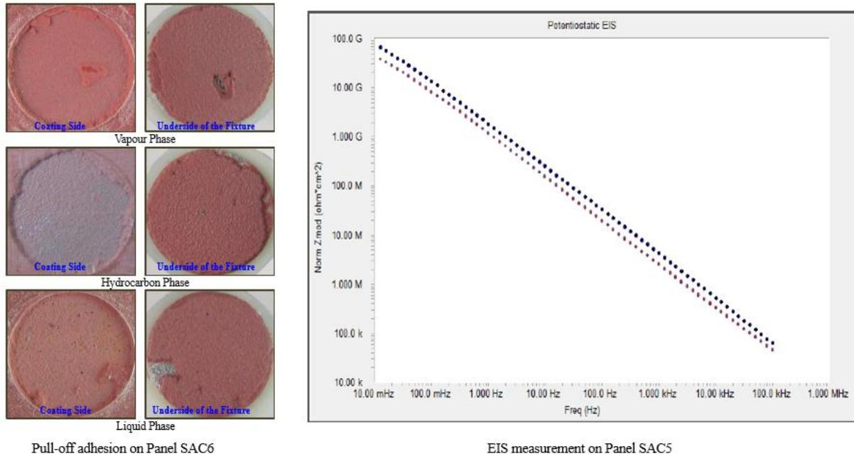
**Figure 8: Pull-off Adhesion Test and EIS Measurements on the 6-Month Standard Atlas Cell Tested Panels of Epoxy Storage Coating System after Curing for 8 Days.**
