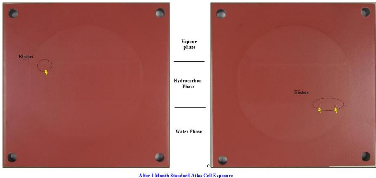
**Figure 6: Standard Atlas Cell Test of the Applied Tankguard Storage Coating System after Curing for 8 Days.**
