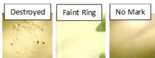
Figure 3 36 Day 50% H 2 SO 4 exposure, Left, PE coating no TMCD, middle the same resin with partial replacement of the glycol by TMCD, right, 100% of the glycol replaced by TMCD
