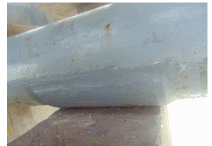
Crevice corrosion of pipes support
