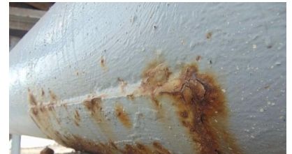
Crevice corrosion of pipes support
