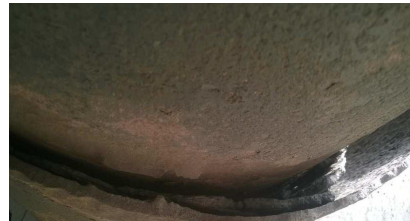
Crevice corrosion of pipes support
