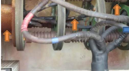
Probable cause of Earlier Failure : Tracking between slip ring body & bare / SS box .
