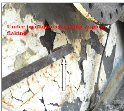
Identification of under insulation corrosion
