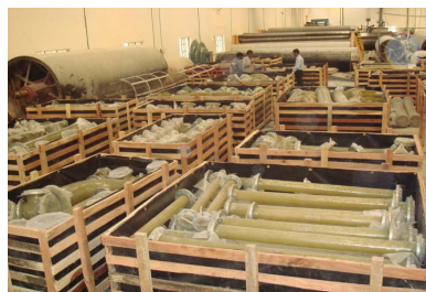
Figure 12: Effluents water and gypsum sludge pipes and fittings for phosphoric acid at 95°C (203°F) in Jordan
