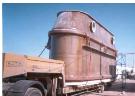
Figure 9: Acid Digester Fume Outlet Fabricated in various shapes with stiffening structures, Morocco.
