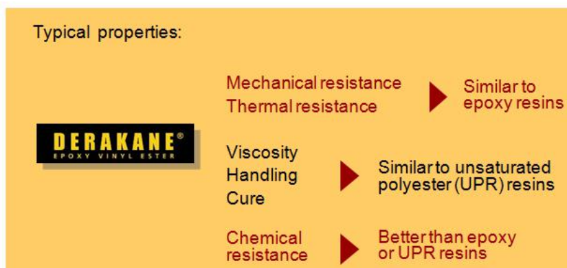
Figure 2. Characteristics of chemical resistant Epoxy Vinyl Ester Resins
