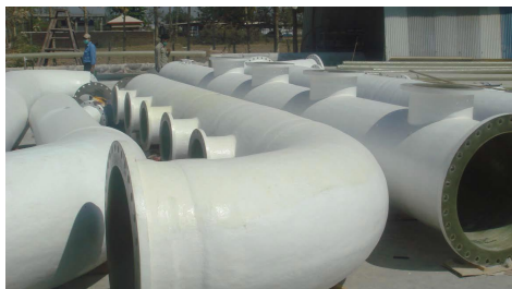
Figure 11: FRP Pipes and fittings for phosphoric acid (46- 54% concentration) at 80°C (180°F) in India
