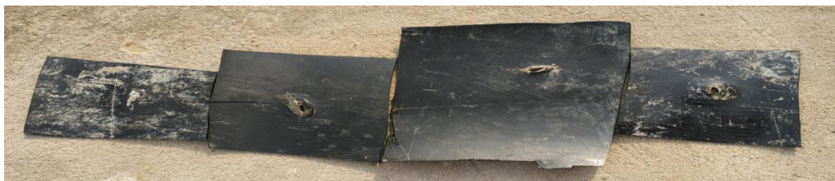
External defect of 52% metal loss
