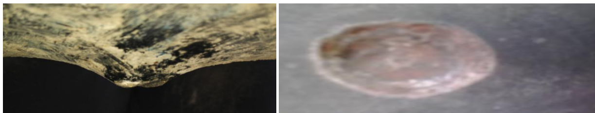
External defect of 52% metal loss
