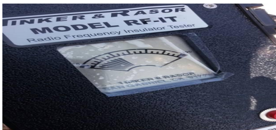
Figure 3: RF-IT shows IJ at Dispatch terminal A was partially short and conducting.
