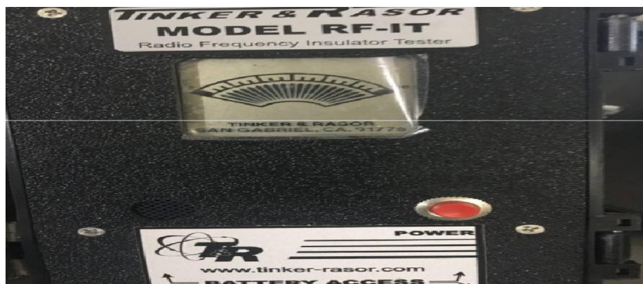
Figure 2: RF-IT shows IJ at Dispatch terminal B was Isolated and Healthy
