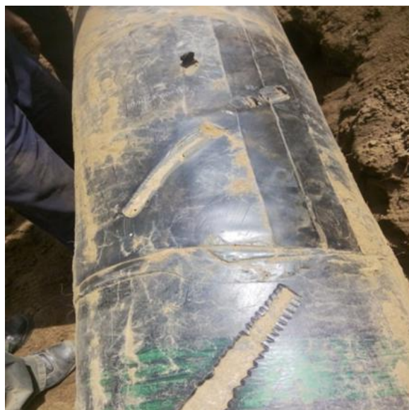
Fig.- 4 Coating & pipe damage at Ch. 617.550 Fig.-5 Coating & pipe damage at Ch. 617.600
