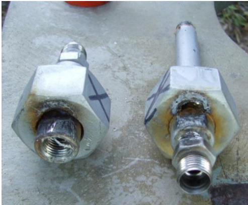
Figure 2. AC fault damage on unprotected isolation unions
