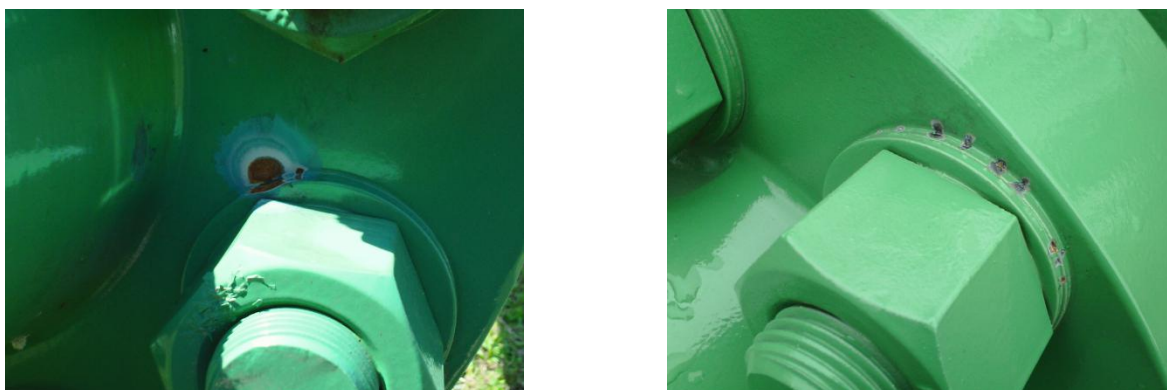
Figure 1. Lightning damage on an unprotected isolation flange
